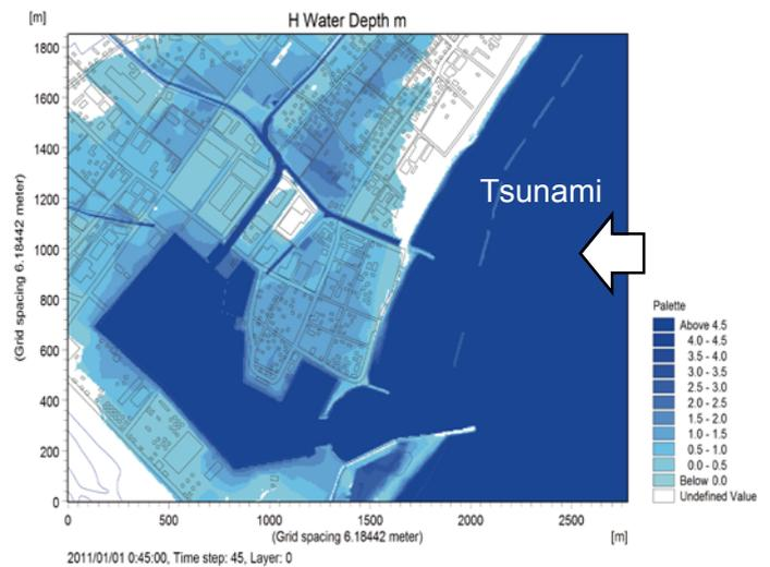
Example of tsunami flooding analysis
