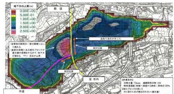
Distribution map of the rise in the groundwater level due to rainfall (After construction)
