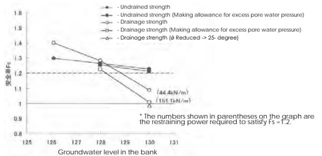
Relation between the groundwater level in the slope and the safety factor
