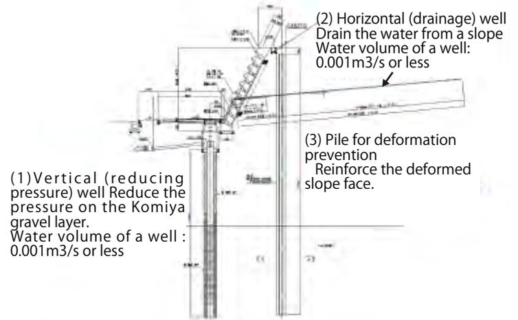
Cross-section of the construction to be conducted as countermeasure
