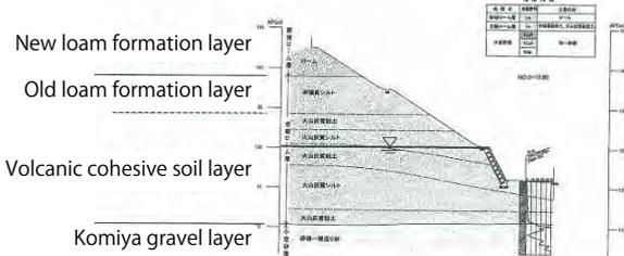
Fig. Soil constants and cross section
